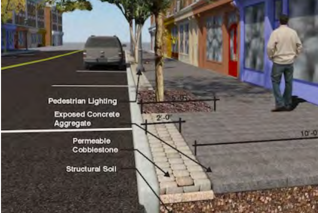
NYACK SIDEWALK IMPROVEMENTS
