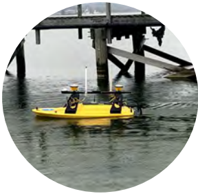
SHALLOW WATER Z-BOAT MULTIBEAM SURVEY
